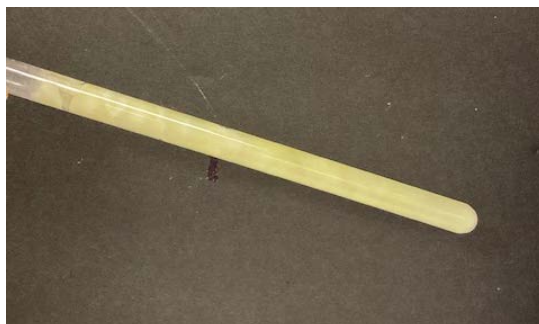
Figure 1. Photograph of \text{CaCl}_2 \cdot 6\text{H}_2\text{O}/\text{SrCl}_2 \cdot 6\text{H}_2\text{O}/\text{PVP} hydrogel composite in a test tube
