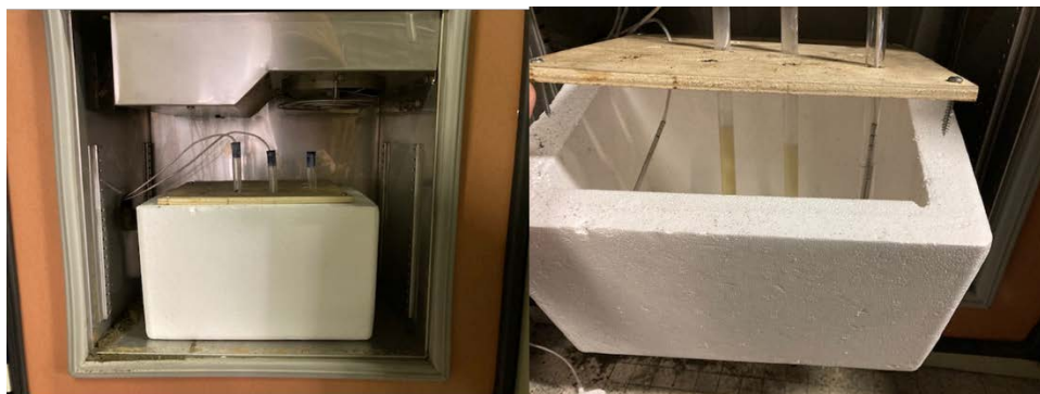
Figure 4. T-history samples setup in a benchtop environmental chamber; Samples were kept inside an insulation box to reduce the rate of heat transfer from the sample to ambient
